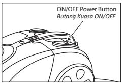
Switch on the power supply and press the ON/OFF Power Button (1) to start operating the vacuum cleaner.
