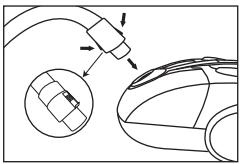
Insert the Hose Connector (4) to the Vacuum Body (12) until it clicks (to release the flexible hose, press the two latches on the hose connector and take it out).
