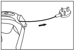
Pull out the Supply Cord to its full length and plug it into the power supply.
