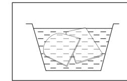
Soak the filter with water, squeeze the water out, then hang it in a shady spot until it is completely dry.
