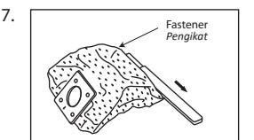
Open the Fastener and dispose of the dirt.
