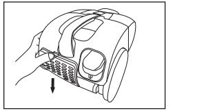
Press the clip down and remove the filter cover by hand.
