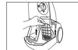
Remove the filter by pulling up the inlet filter cover.
