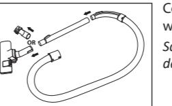
Connect the Flexible Hose Handle (10) to the Floor Brush (7) (or Dusting Brush with Nozzle) together with Telescopic Tube (9).
